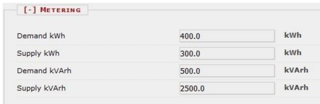
Figure 1-1 Measured values of the metering function
